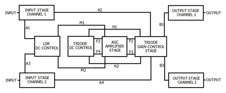
FIGURE 8 ALL TRIODE PROCESSOR BLOCK DIAGRAM
